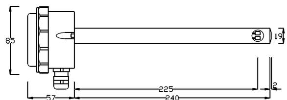
Note: each unit is supplied with a foam gasket 3mm thick before compression
